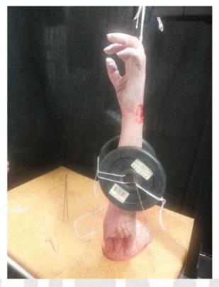
**Fig. 2** Cadaver is suspended; forearm bones are blocked in neutral rotation, Elbow is secured manually.
